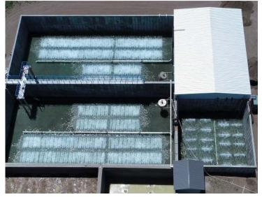
One 2m long OxyStrip™ is equal to 9 times 9" disc Installation
