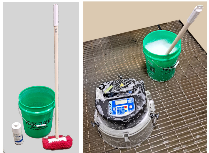
Figure 12. (a) Cleaning supplies: detergent, brush with polyolefin bristles, HDPE plastic bucket, and 6712 top cover. (b) Cleaning the Teledyne ISCO 6712 top cover.
